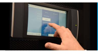
Delta's DPH series Modulon UPS offers the ability to view up to 10,000 event logs on the touch panel. The unit's 10" LCD screen can optionally display information on security, cooling, fire protection, and temperature in addition to battery status. The availability of all this information on the touchscreen of the UPS allows for easy local management.
